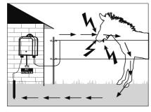
The energiser may be used outdoors only in conjunction with an electric fence to keep animals in/out as required.
